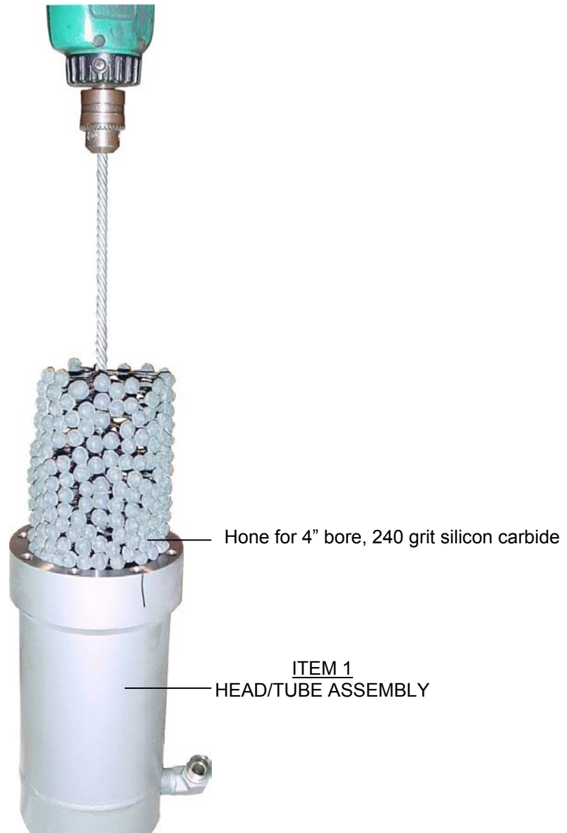
FIGURE 14 CLEANING THE HEAD/TUBE ASSEMBLY
