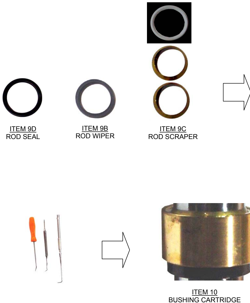
FIGURE 20 REINSTALLING THE ROD SEAL, WIPER AND SCRAPER
